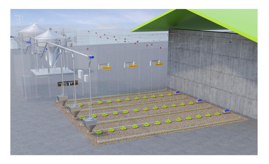
TEXHA has designed the comprehensive solution and offers ready-to-use sets of processing equipment with automated control of the poultry life support processes, including feeding, drinking, lighting and microclimate.
